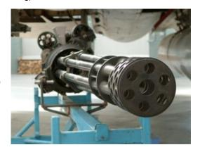
because of its multiple barrel configurations it has a jam rate less than 1 in 10,000.
